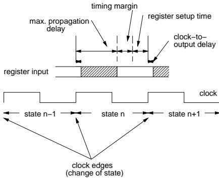
Using a single clock means we only need to compute the delay through *combinational* logic blocks which is much simpler than having to deal with asynchronous clocks. This is why almost all large-scale digital circuits are synchronous designs.
