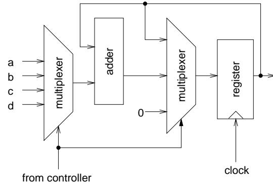
Exercise: Other datapaths could compute the same result. Draw the block diagram of a datapath capable of computing the sum of the four numbers in three clock cycles.
